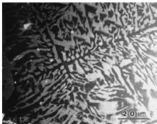
Figure 6 Optical photograph of the directionally solidified \text{BaTiO}_3 - \text{CoFe}_2\text{O}_4 eutectic grown under conditions of a growth rate of 20 mm/h in 2.5% \text{O}_2 in \text{N}_2 .
